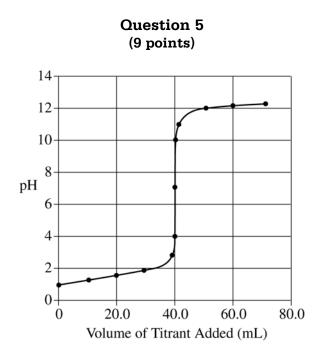
A solution of 0.100 M HCl and a solution of 0.100 M NaOH are prepared. A 40.0 mL sample of one of the solutions is added to a beaker and then titrated with the other solution. A pH electrode is used to obtain the data that are plotted in the titration curve shown above.
